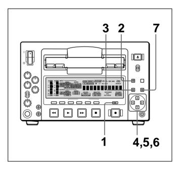
1 Press the COUNTER SELECT button to light the time data type indicator "TC" or "U-BIT."
